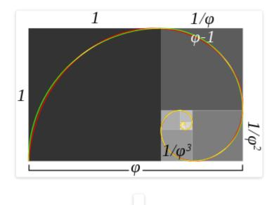
Approximate and true golden spirals. The green spiral is made from quarter-circles tangent to the interior of each square, while the red spiral is a Golden Spiral, a special type of logarithmic spiral. Overlapping portions appear yellow. The length of the side of one square divided by that of the next smaller square is the golden ratio.
